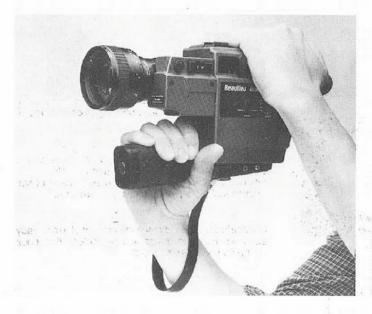
The picture above shows how you should hold the camera when filming. You power and release the camera with your right hand. The strap around your wrist will avoid accidentally dropping the camera.
