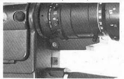
rotate the front ring until the distance index faces upwards. Then frame a subject with vertical lines (e.g. a building) and improve the picture adjustment by making lines appear vertical in the viewfinder.
