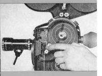
retaining screws should only be loosely tightened.
