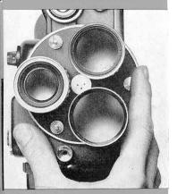
locking catch, thus freeing it (27). To swivel the turret (either clockwise or antichlockwise), use the three knobs fitted between the lenses, to avoid any risk of modifying their settings. Once the catch has clicked into place, the lens chosen for filming is properly aligned (upper position) (28).
