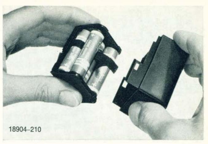
lifting the upper (slightly bent) edge of the metal lid from its catch and separate both
