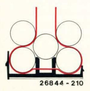
parts. Insert each cell in its retaining clip observing + and - polarity. Place the end of the cell against the spring contact and push it into the clip. The fabric bands are placed beneath the lower cells to facilitate their removal. Close the battery housing.
