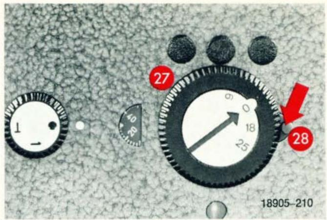
Insert battery housing (1) into the camera by engaging its upper portion with the spring clip in the camera body. Tilt the housing downward until it is secured. Test the battery by setting frame speed selector (27) to any speed and then depressing locking button (28). The needle of battery test indicator (2) should be in the white sector. If the needle remains in the red sector, the batteries are exhausted and should be replaced.
